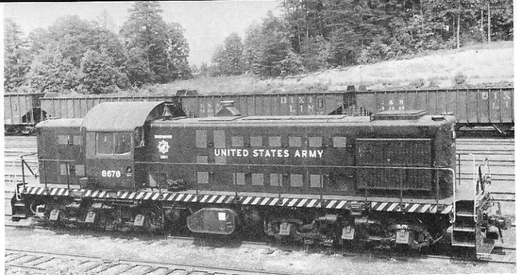
Ken Douglas USA #8678, later r# TVA #42, on TVA property at Kingston, TN, 26May72 shows top detail, offset stack, etc., of typical RSD1. None of the 8600's had numberboards while all the 8000's did. Also 8600's were 131-ton Spec. E1646, while 8000's were 127-ton Spec. E1645.
