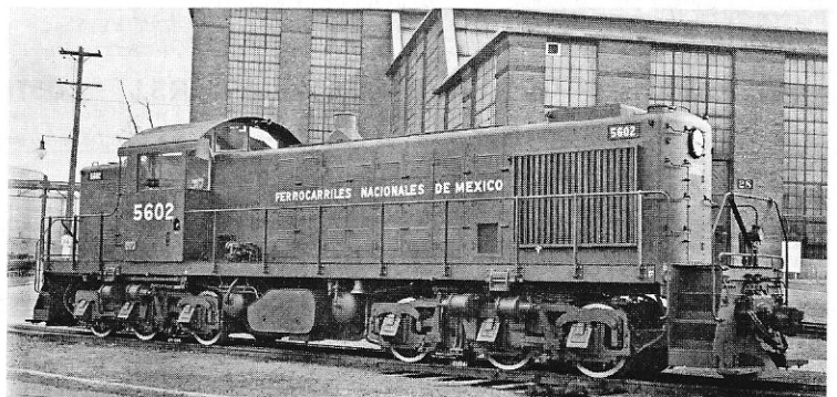
Alco Historic Photos NdeM RSD1's (E1647) #5600-05 (r# 5700-05) were very similar to USA 8600's except for having standard cabs and numberboards, and were the last of 163 RSD1's built. Unusual truck design, peculiar to RSD1's, was a fabricated, equalized, rigid bolster, pedestal type apparently designed and built almost "overnight" for the rush Trans-Iranian program in L/1942, maybe by James G. Blunt (Blunt truck) in charge of Alco engineering then.
