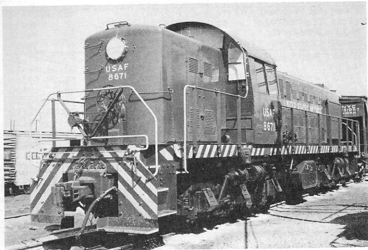
Don Dover Detail end view shows slant to export cab sides, brake wheel, mu (on all RSD1's except #8000-07). Plug on cab step is for undercab fuel tank drain. At least 12 RSD1's were at sometime lettered USAF: 8007, 10, 12, 14, 33, 50; 8656, 60, 62, 66, 71, 72. USAF 8671 at Sharon Yard (Cincinnati), OH, E10/68, en route to Eglin AFB, FL.
